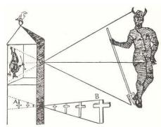
The dark room allows to observe in a surface the reflection of the external phenomena. The images are ephemeral, they are light that can not be retained.
